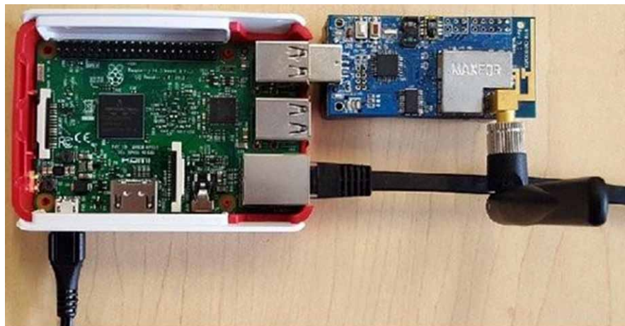
Figure 5. RaspberryPi 3 with the TmoteSky sink mote (Kamgueu et al., 2017).
