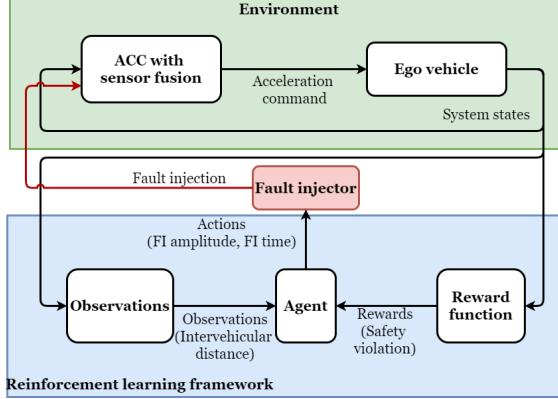
Figure 5: Connecting reinforcement learning, fault injection, and the environment
