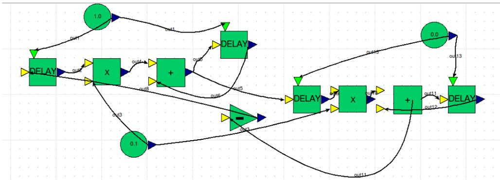
Figure 6: The circle test as implemented in a causal block diagram
